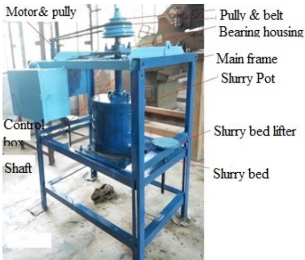
Fig.2 Erosion pot tester (experimental setup)
