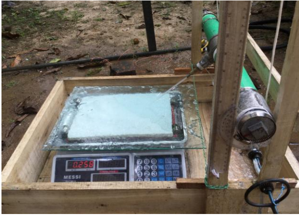
Fig.2 A cleaning method of a glass plate as a glazing material
