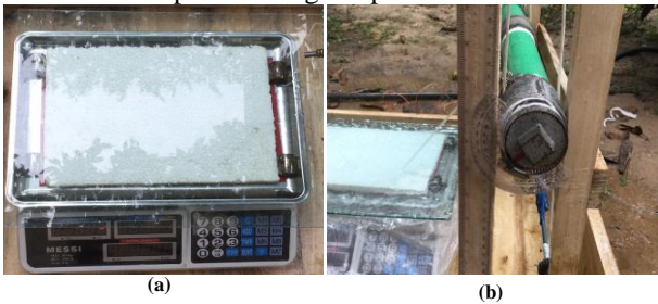
Fig. 3 (a) Weight measuring device with glass plate and roller; (b) Angular and vertical position measurement
