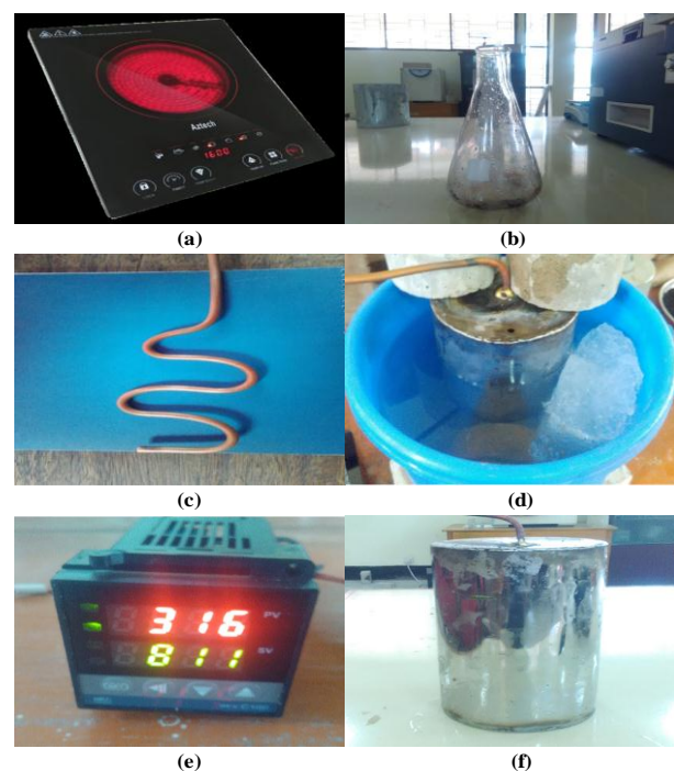
Fig. 1 (a)Infrared Cooker;(b)Conical flask; (c)Copper tube; (d) Ice bath; (e)Temperature monitor; (f)Stainless steel cylinder.
