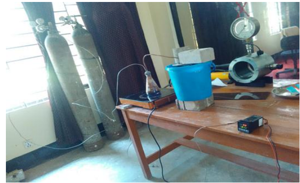
Fig. 3 Photograph of sawdust pyrolysis process
