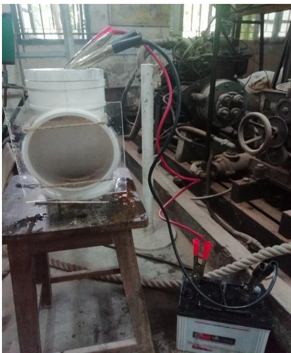
Fig 4 : Experimental Setup of HHO Gas Generator
