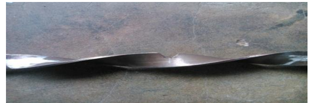
Fig. 4: V-shaped twisted tape insert of stainless steel
