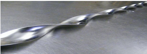
Fig. 1: Twisted tape insert without any cut
