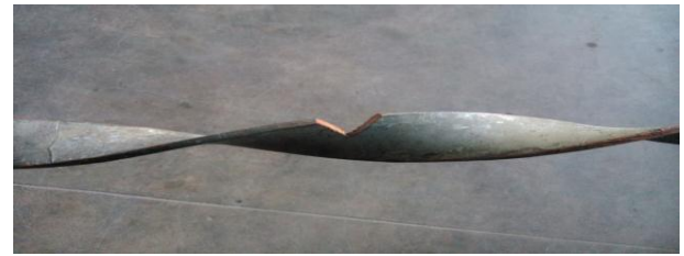
Fig. 3: V-shaped twisted tape insert of copper
