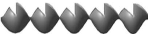
Fig. 2: Twisted tape insert with V-cut
