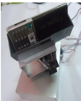
Fig. 5: Pan-tilt allocation system with camera
