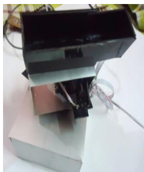
Fig. 4: Pan-tilt allocation system without camera
