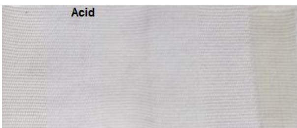
Picture:4- Color fastness to perspiration in acidic medium.
