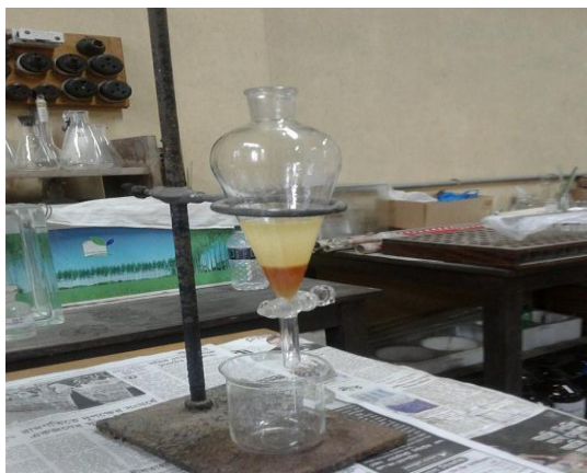
Fig. 3 Separation process in separating funnel
