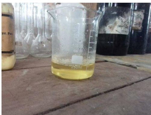
Fig. 4 Extracted biodiesel after separation
