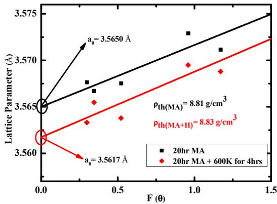
Figure 3: Lattice parameters of as milled and annealed samples.
