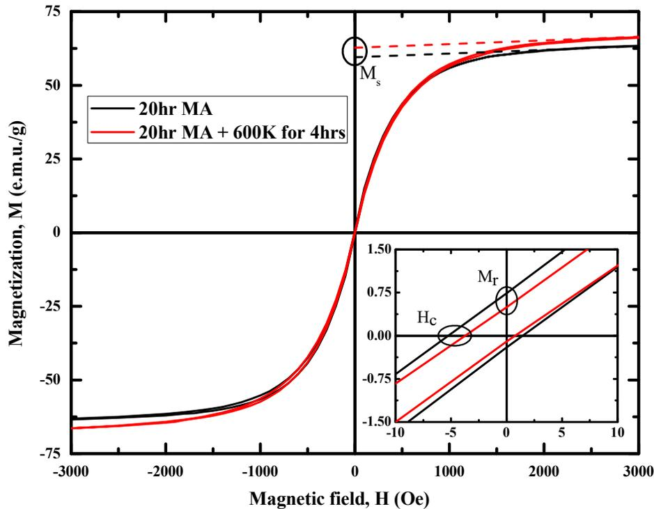
**Figure 7:** M-H loop of the as milled and annealed samples.
