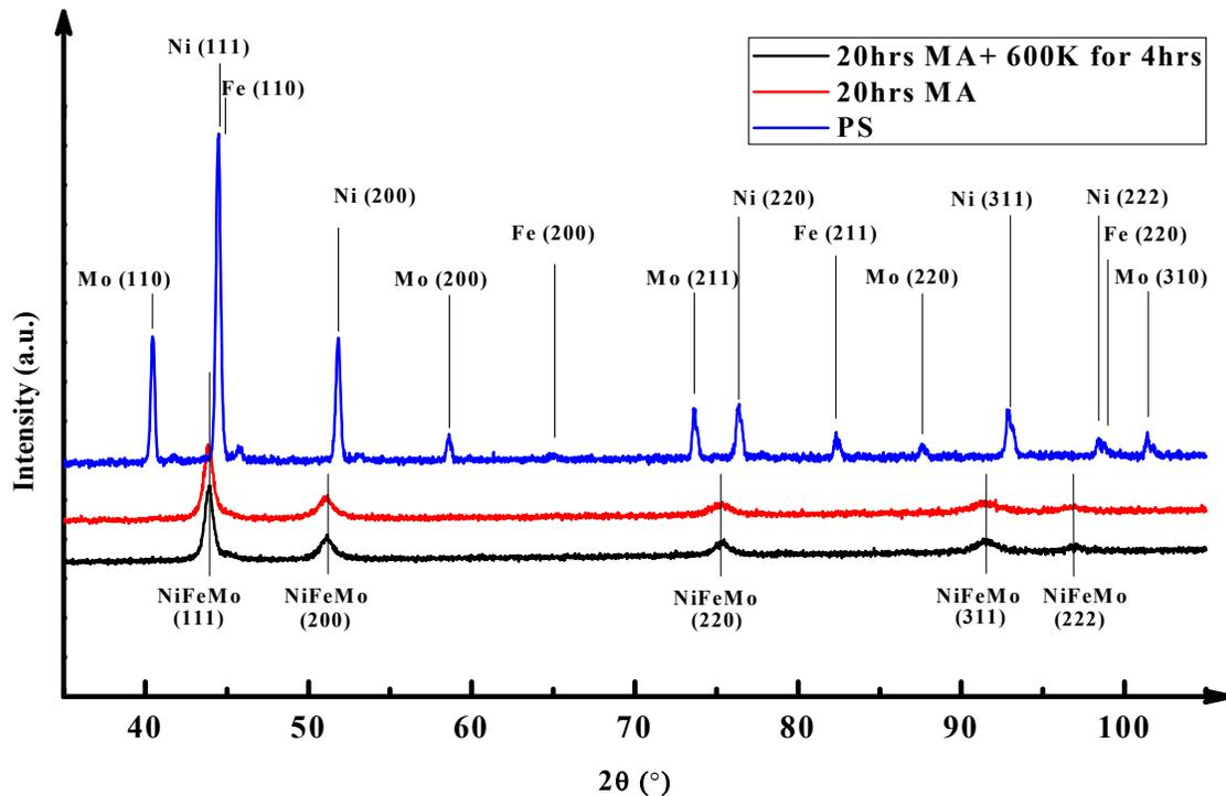
**Figure 1:** XRD patterns of PS, 20hrs milled and 20hrs milled plus annealed samples.
