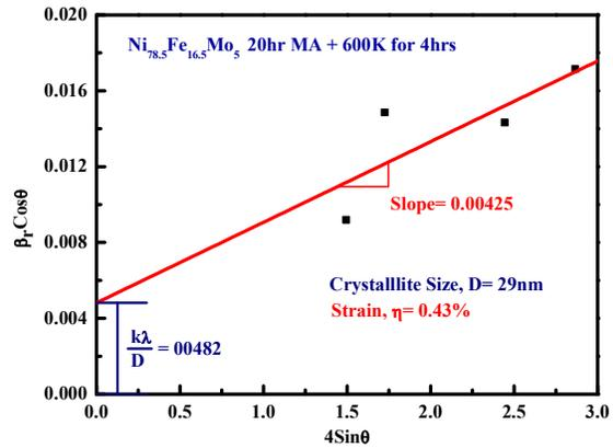
Figure 4: Crystallite size and micro-strain of the alloy.
