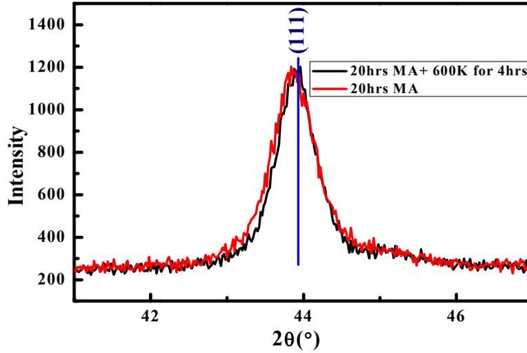
Figure 2: XRD patterns with an exact intensity of 20hrs as milled and milled plus annealed samples.
