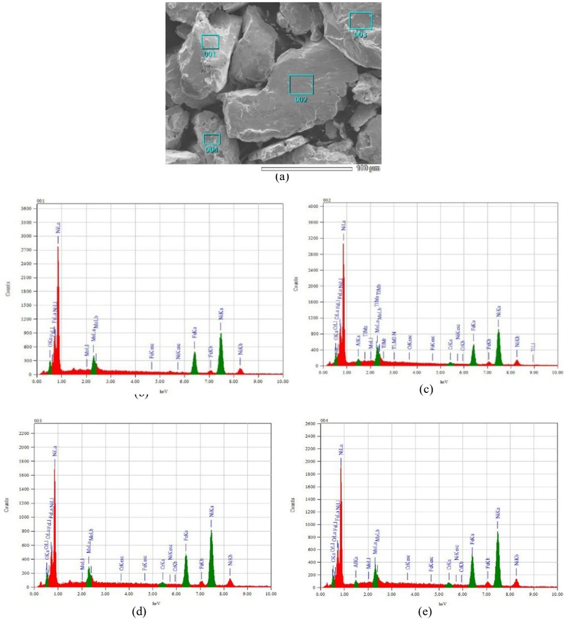
**Figure 6:** EDX-analysis for different points, (a) position of points, (b) counts for point 1, (c) point 2, (d) point 3 and (e) point 4.
