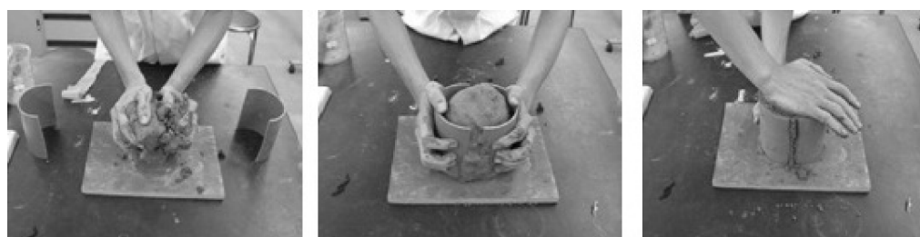
Figure 4 Shaping of Filter from Dough Using Dice
