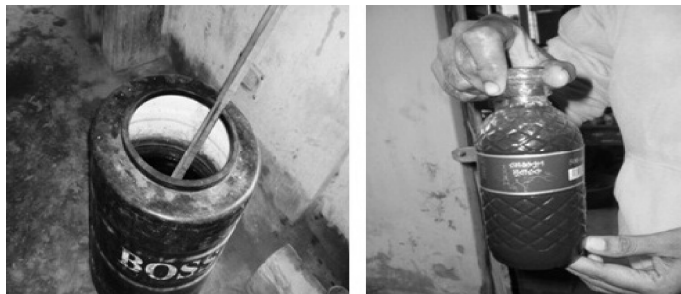
Figure 10 Iron Bacteria Culturing and Collected Iron Bacteria Sludge.
