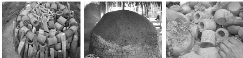
Figure 7 Filter Burning in Potter Kiln
