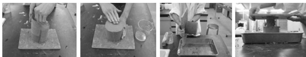
Figure 5 Final Step to Get Raw Ceramic Filter
