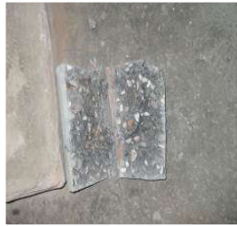
Figure 16 Brittle failure of specimen T 1
