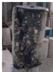
Figure 12 Brittle failure of specimen C 1
