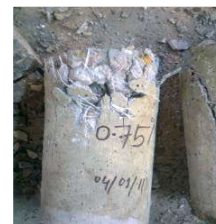
Figure 14 De-bonding of fiber-matrix of specimen C 4
