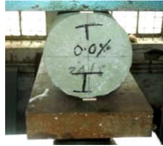
Figure 10 Test set up for splitting tensile strength
