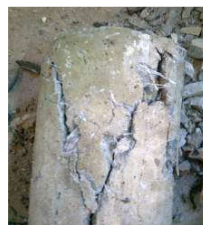
Figure 13 Wedge failure were observed in specimen C 2 and C 3
