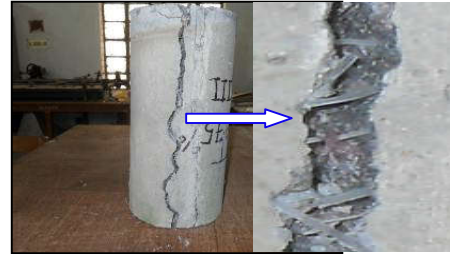
Figure 17 Fiber bridging of specimens T 2 , T 3 and T 4
