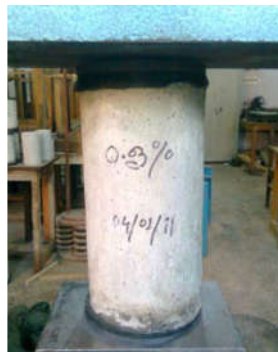
Figure 8 Instrumentation of cylinder specimen to test the compressive strength
