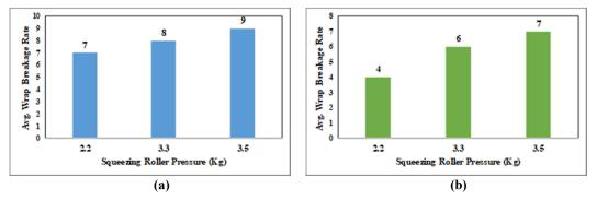
Figure 3: Varying squeezing roller pressure and their effect on the average warp breakage rate (a) for shift A and (b) for shift C.
