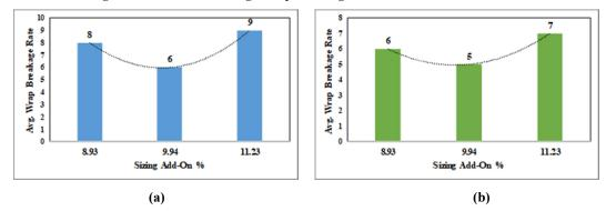
Figure 1: Different sizing add-on% and their impact on the average warp breakage rate (a) for shift A and (b) for shift C.
