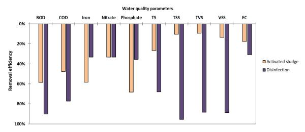
Figure 8: Comparative Chart of the Removal Efficiencies in Activated Sludge Treatment Unit Followed by Up-Flow Duel-Media Granular Filter Unit.
