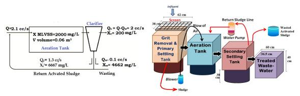
Figure 3: Process Variables (left) and Schematics (right) of Activated Sludge Treatment Unit.
