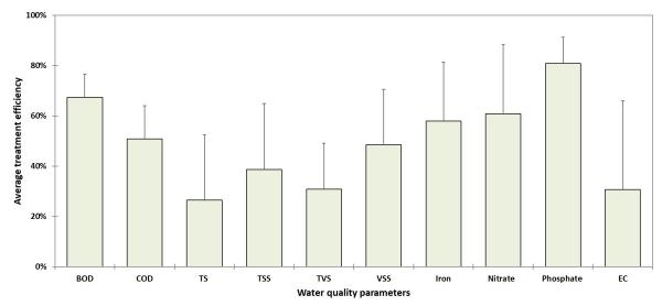
Figure 7: Average Treatment Efficiencies in the Developed Activated Sludge Treatment Unit.
