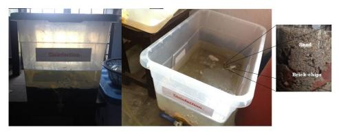
Figure 6: The Developed Upgraded Duel-Media Filtration Unit.
