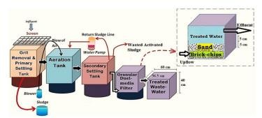
Figure 5: Schematics of the Upgraded Duel-Media Granular Filtration Unit.
