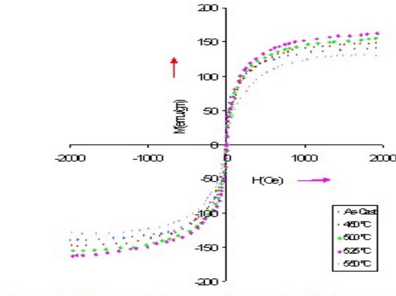
**Figure 3:** Magnetization of Sample-A at as-cast and different annealing temperature
