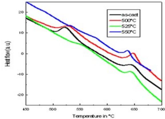
**Figure 2:** DTA analysis of sample-B at as-cast and different annealing temperature
