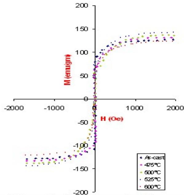
**Figure 4:** Magnetization of Sample-B at as-cast and different annealing temperature
