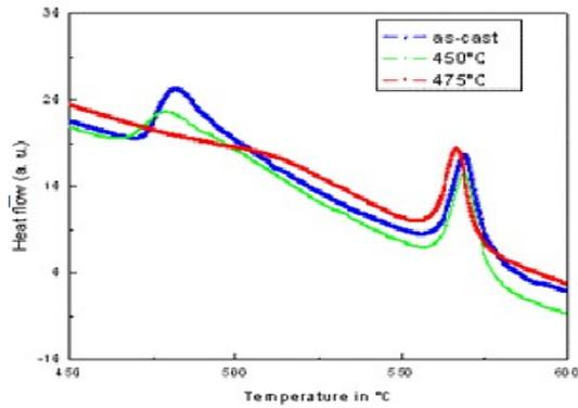
**Figure 1:** DTA analysis of sample-A at as-cast and different annealing temperature
