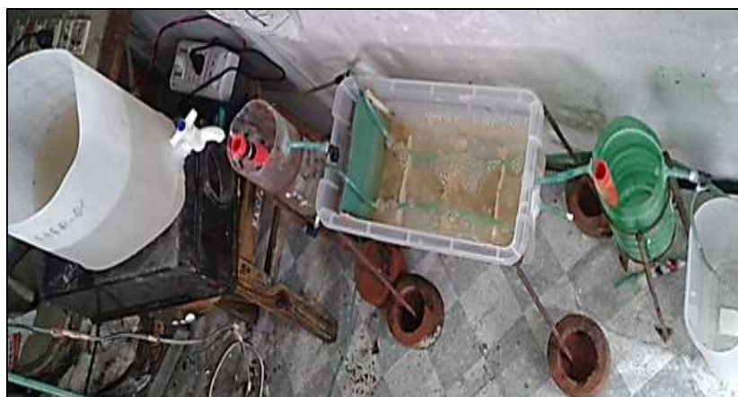
Figure 6: The bench scale biological wastewater treatment plant
