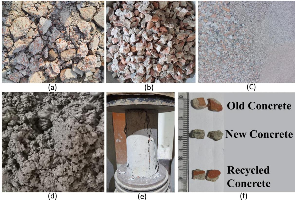
**Figure 1:** (a) Old demolished concrete, (b) Recycled Coarse Aggregate (c) Recycled Fine Aggregate (d)
